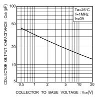
Fig.8 Collector output capacitance vs. collector-base voltage
