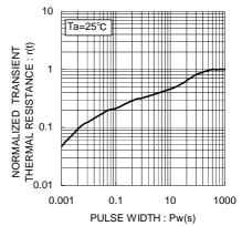
Fig.9 Normalized thermal resistance (Element)
