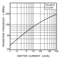
Fig.7 Gain bandwidth product vs. emitter current
