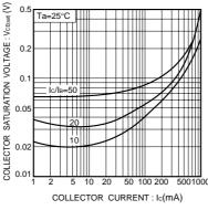
Fig.5 Collector-emitter saturation voltage vs. collector current ( I )
