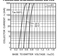
Fig.1 Grounded emitter propagation characteristics
