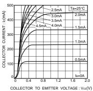
Fig.2 Grounded emitter output characteristics
